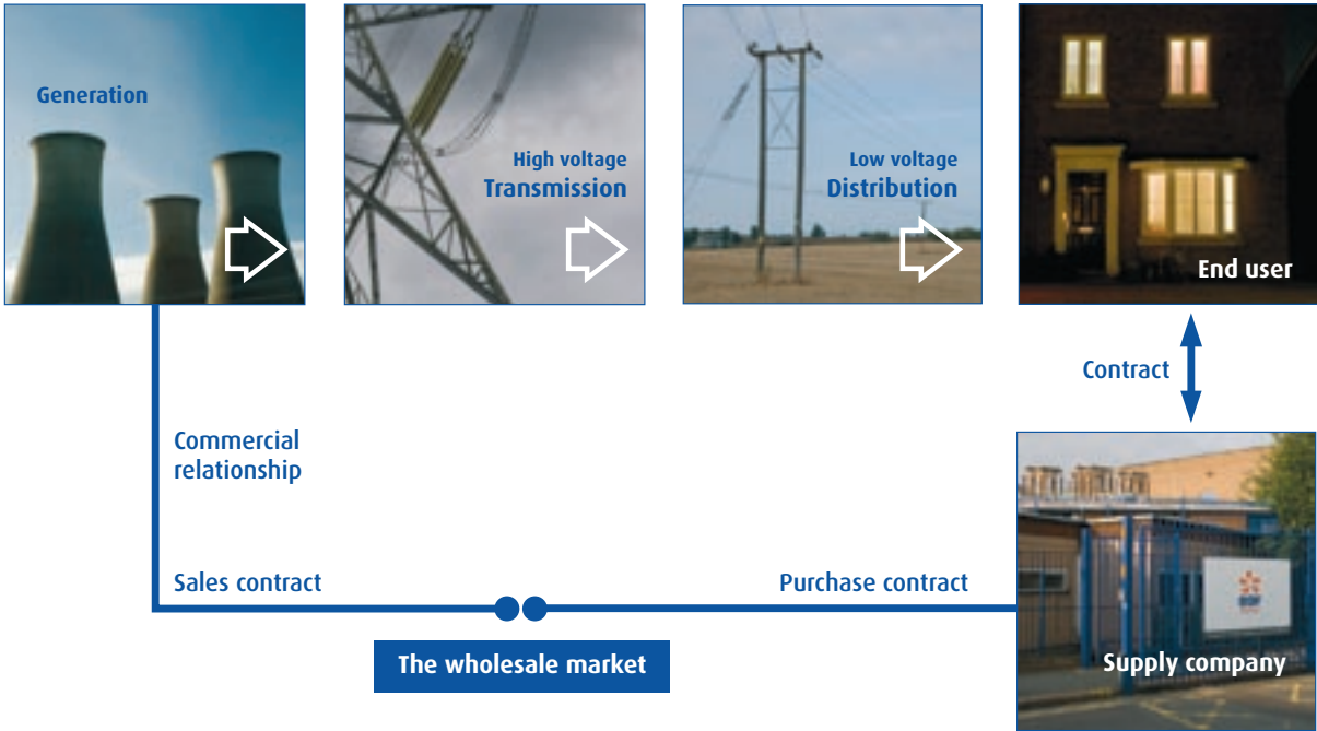
Figure 2 Technical flow of electricity
